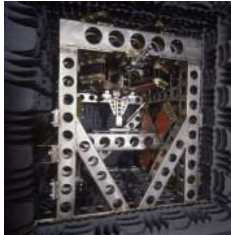
Instrument used for positioning & moving specimens plus for measuring friction & normal forces
