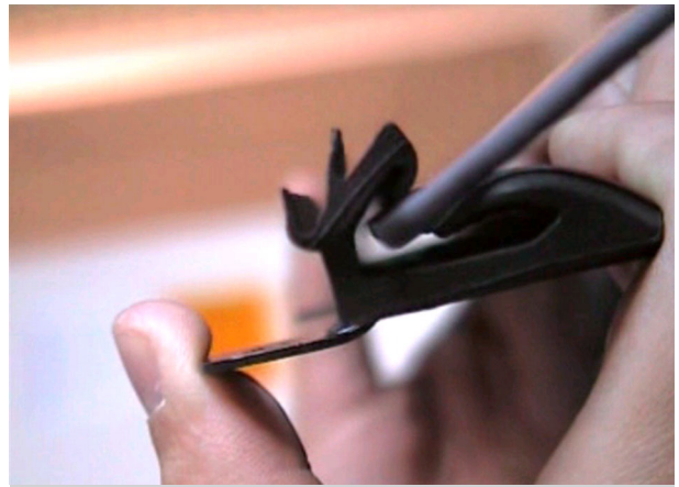
Fig. 6: critical contact glass plate to door sealing
