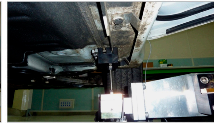
Left Rear shock tower control accelerometer
