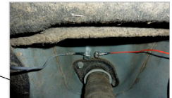
Left Rear shock tower control accelerometer
