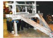
Vertical, Fore-Aft and Pitch motions, controlled on Cross Car Beam in vertical direction; 2 ED shakers driven in-phase
