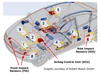
Airbag control units (ECUs) in advanced airbag systems process multiple sensor inputs to determine the type and severity of a crash plus occupants' restraint, size, weight, and position. The ECU decides which multiple airbags to deploy and with how much force.
