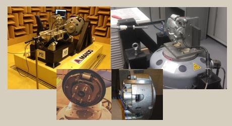
MB Brake Rattle Detector is a quiet, non-hydraulic lab test system that subjects brake assemblies and components to invehicle vibrations sequentially in multiple directions.
