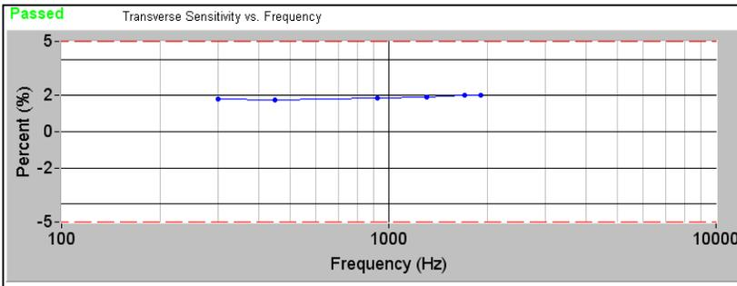
Typical plot created by Win475 software showing one measurement at each frequency step for S/N 1685 (see Reproducibility table above). All data collected at 10 g's peak, nominally 100 m/s<sup>2</sup> of vibration amplitude. Frequency range available is 30 Hz to 2000 Hz at 10 g's. Data were also collected at 15 g's and 20 g's peak with no apparent improvement in signal-to-noise or reduction in measurement uncertainty.
