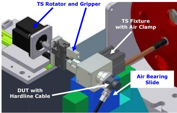
The Win475-TS Measurement Option for MB's Win475 Automated Vibration Transducer Calibration System transforms accelerometer transverse sensitivity measurement because it measures at multiple, user-selectable frequencies – low frequencies for servo, seismic and modal accelerometers; higher frequencies for general-purpose sensors. Frequency-response plots show how the transverse sensitivity amplitude varies.
