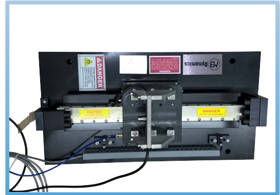
Horizontal Excitation MB CAL2-300H Exciter for \leq 5 kg Payloads with 280 mm Stroke (300 mm between stops)
