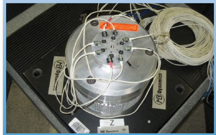
Win475 MDCC mounted with eight (8) piezoresistive accelerometers
