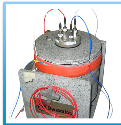
"4-in-1" MDAC mounted with four (4) PE accelerometers
